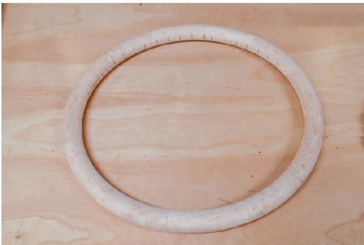
Roger Wayman shows us the segmented wooden steering wheel that he made for a friend's classic car
