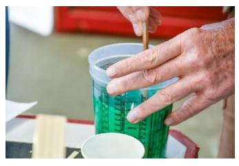
catalyst are heated after mixing, it will speed up the curing process.
