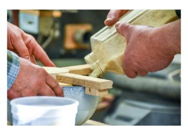
Using rice to measure the volume of the mold
