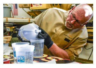
Resin and catalyst can be made thinner and easier to work with if they are gently heated *before* mixing, 120 F is a good temperature for this. Wayne uses a pizza oven in his shop to heat the jugs holding the resin and catalyst. However, if the resin and
