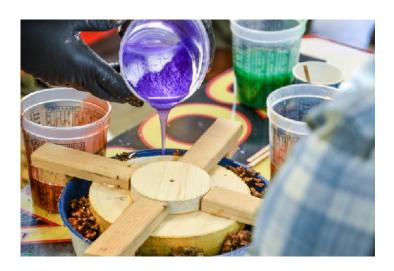
use for a project, especially if you are coloring the resin. So, Wayne uses a mold filler for bowl castings to fill up some of the space which will be turned away when the bowl is finished on a lathe. For this project the mold filler was a hardwood hemisphere, coated so it would not soak up any of the resin, and attached to a jig which would hold it centered in the bowl mold.
