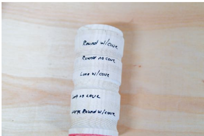
Examples of effects with different burrs and shapes
