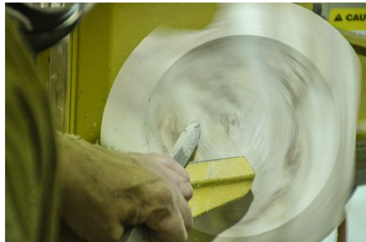
Making the finishing cuts.
