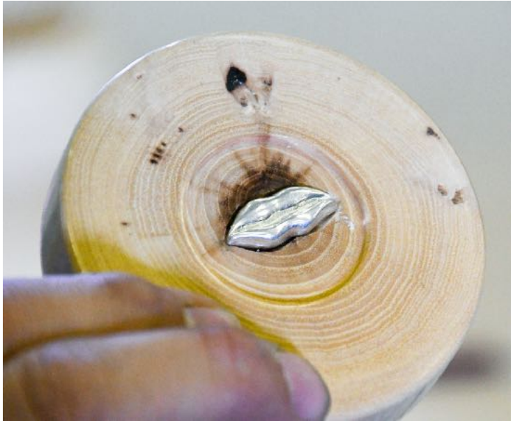
The final fit. The insert is then epoxied in and finished with polish.
