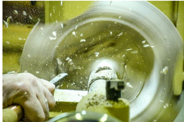
After sanding, the blank is reversed and the bowl is hollowed out.
